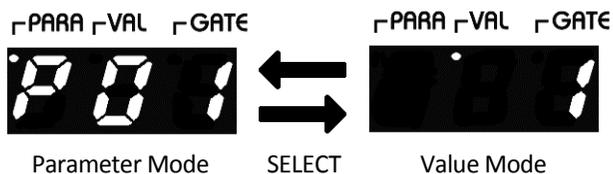
When the PRO SOLO Mk3 is in Parameter Mode, the PARA dot will be lit and “P” will appear in the left digit. The parameter number will be shown in the right two digits. An overview of the parameter list is printed on the PRO SOLO Mk3 itself, although whenever the parameter number is changed, its name will scroll across the display – i.e. “MIDI rec channel”. The full list of parameters and their associated values can be found starting at page 14.
